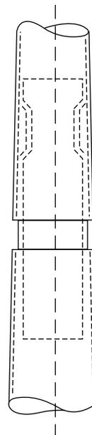
All shafts with overall length of 33' or more are shipped in **two sections**
